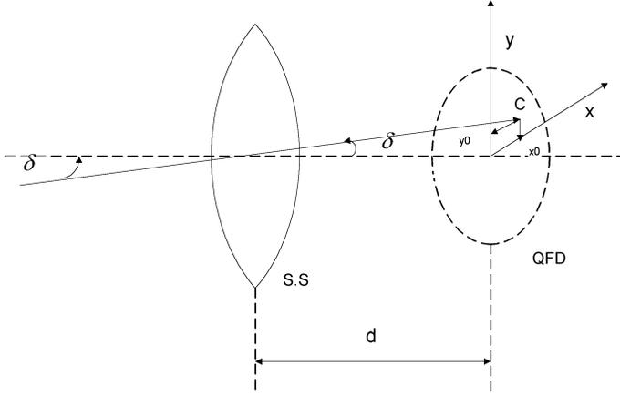
Fig. 2. Geometry between thin lens and quadrant photodiode
