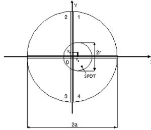
Fig. 3. A spot position on quadrant photodiode surface
