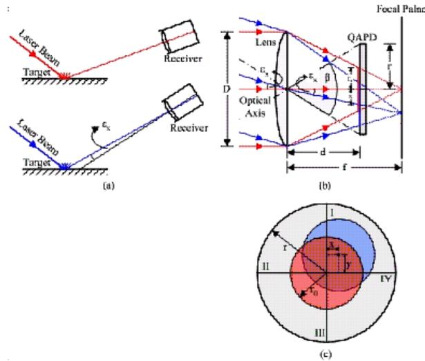
Fig. 1. Laser beam and receiver of reflected laser beam
